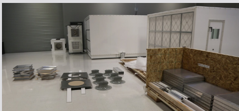
Disassembled Knock-down FANWALL Cube, ready for crating
