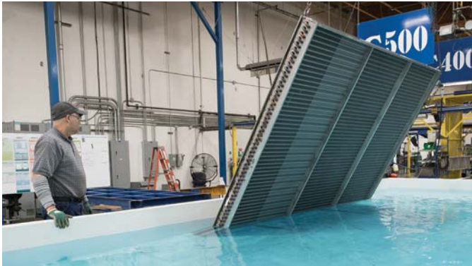
Every coil is submerged in a tank of water and pressurized with dry air to check for leaks.
