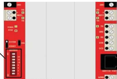
Figure C7: BacNet address jumpers
