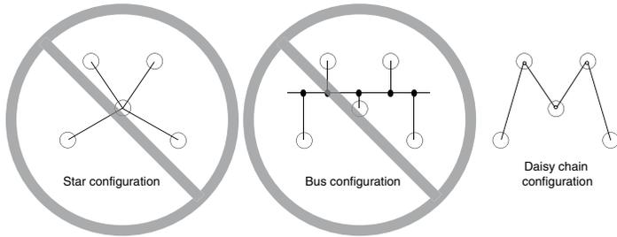
Figure C2: Network configurations – star, bus and daisy chain
