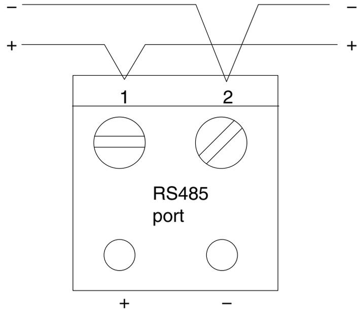
Figure C3: Proper connection in the middle of a daisy chain
