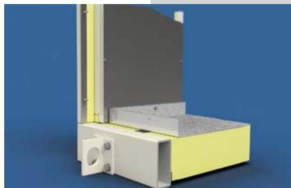
Inferior thermal break design with liners moved to exterior of panels.
