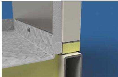
Z-bar is tack welded and caulked – NOT continuously welded. Water leak potential. Z-bar is a thermal bridge.
