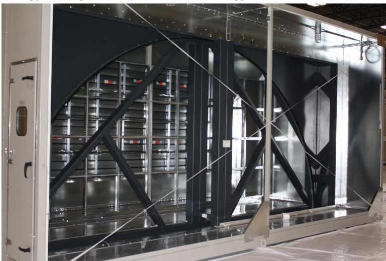
20-foot diameter energy recovery wheels—as big as they get!
